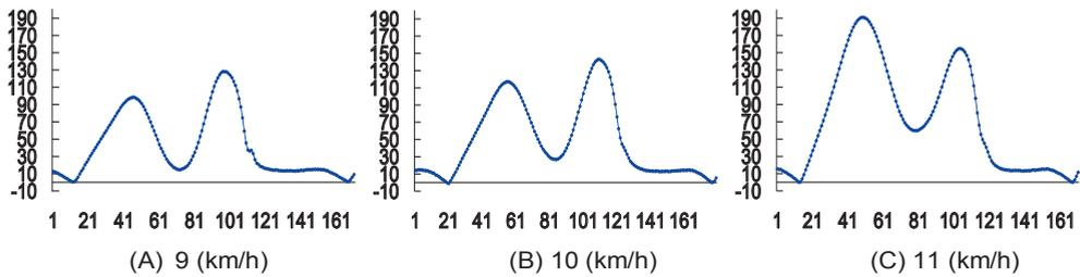
Figure 2: (A)(B)(C) are the toe height at three speeds. The first peak toe height increased with treadmill speeds. The ordinate axis show the height of toe in millimeter. The cross axis show the time in millisecond.
