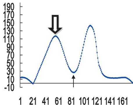
Figure 1: The height of toe in a gait recycle.  $\Downarrow$  Present the first peak  $\Uparrow$  Present TC. The ordinate axis show the height of toe in millimeter. The cross axis show the time in millisecond.
