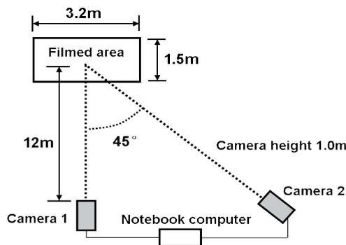
Figure 1: Measurement setup.
