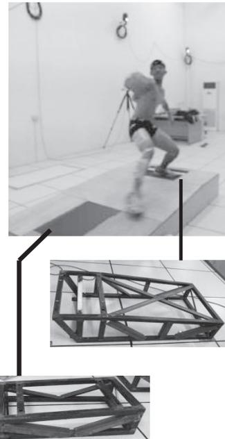
**Figure 1:** The structure of pitching mound. Two force plates were locked on these steel frames, then a wooden box covered it.
