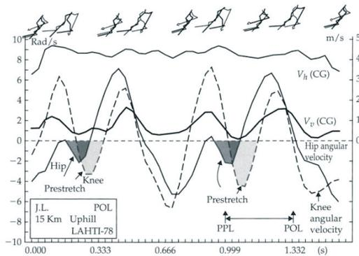
**Figure 1: Horizontal velocity ( $V_h$ ) and vertical velocity ( $V_v$ ) of the body CoG together with the angular velocity curves of the hip and knee. The hatched areas represent the parts of the cycle where the extensor muscles of these joints are assumed to be prestretching (negative velocity) just prior to propulsion extension (positive velocity) (Komi & Norman 1987)**
