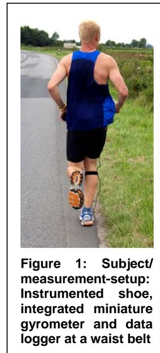
**Figure 1: Subject/ measurement-setup: Instrumented shoe, integrated miniature gyrometer and data logger at a waist belt**
