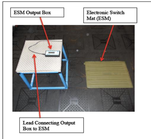
**Figure 1. Electronic switch mat positioned over a force platform.**
