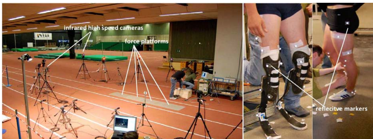
Figure 1. Representation of the experimental setup. Left: Indoor running track, camera system and force plates. Middle and right: Marker placement.
