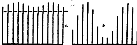
Figure 3: The illustration is the limitation noninformation part of the periodogram and amplify of the information part.
