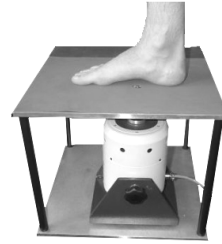
Fig. 3: Detection of vibration thresholds with a Vibration-Exciter.
