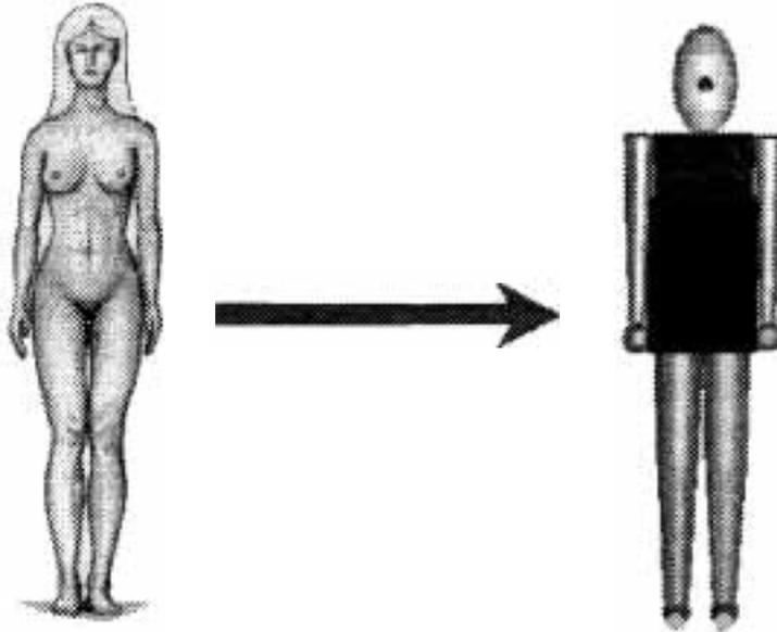
**Figure 1 - Human anatomy projected onto the Hanavan model**
