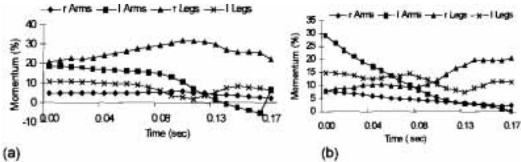
Figure 3 - Percentages of the forward momentum of the arms and legs during the support phase of the one-foot (a) and two-foot (b) back row jump spike
