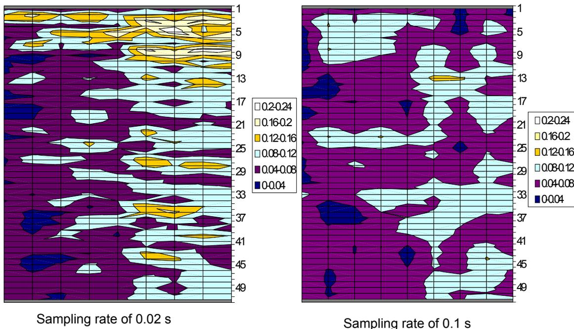
**Figures 5 and 6 - Distances of markers and corresponding points on the model at a sampling rate of 0.02 s and 0.1 s shown in a surface mesh grid.**
