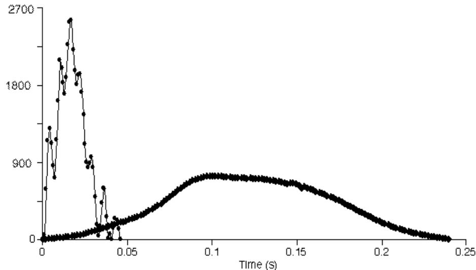
**Figure 1 - Comparison of vertical force (N) in a power drop exercise ( ♦ ) and a direct force platform impact ( • ) for a 6.8 kg MB with a 124 cm drop.**
