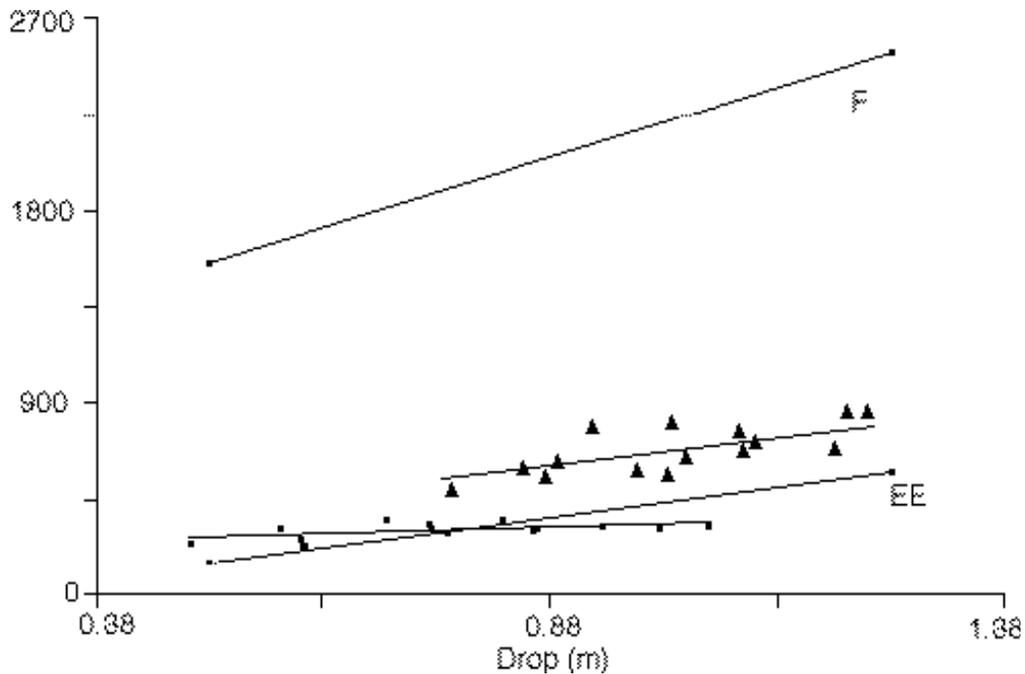
**Figure 2. Scatterplots of the significant ( $p < 0.05$ ) associations between drop height and peak force (N) in a 5.4 kg power drop exercise for a female (·) and a male subject. The corresponding regression lines, the regression line for the direct force platform impacts (F), and the EE are illustrated.**
