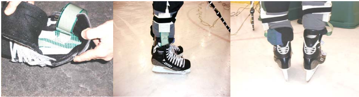
Figure 1 - The top (a), side (b) and rear (c) views of the sensor placement during testing.
