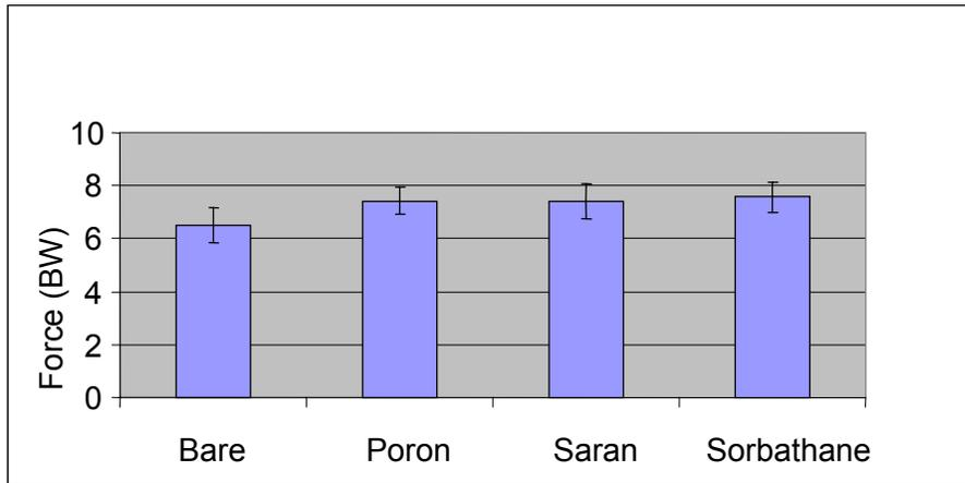
**Figure 2 - Mean ( $\pm$ SE) peak vertical force with different insoles relative to landing barefoot.**
