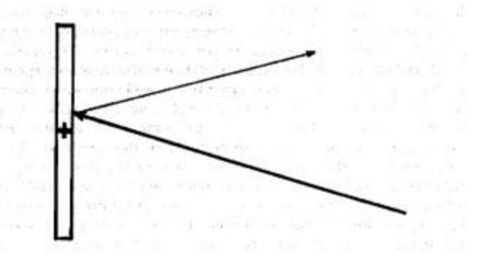
Figure 1. Top view schematic of impact conditions. Lateral deviation of ball rebound in this transverse plane was measured.
