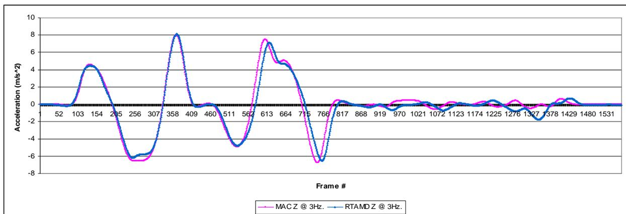
**Figure 1 Comparison graph illustrating difference between acceleration (Z direction) calculated using a motion analysis system (MAC) and the RTAMD**
