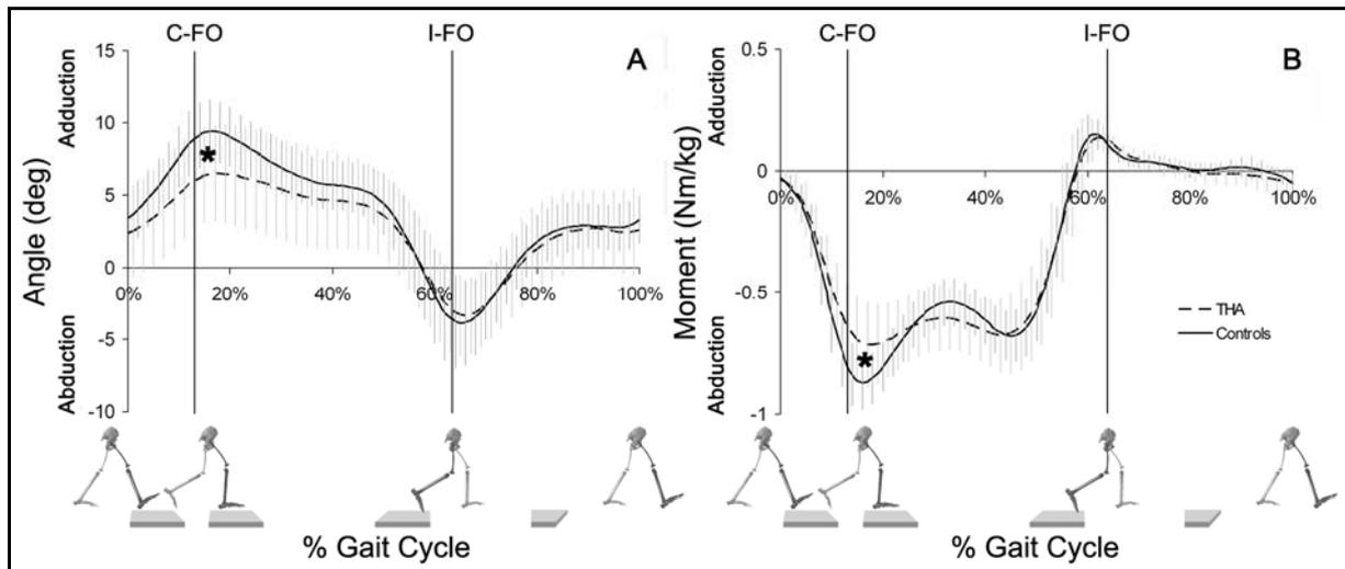
**Figure 1: Average (and standard deviation represented by grey vertical lines) (A) hip angle and (B) hip moment of force in the frontal plane during level walking, time-normalized to the gait cycle. The asterisks (\*) represent statistically significant differences between the THA and control groups.**
