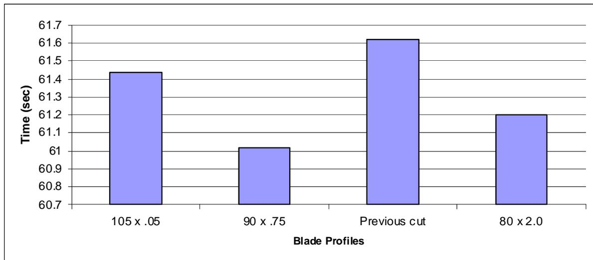
**Figure 2: Shows the total average time to complete all four drills for each blade profile.**
