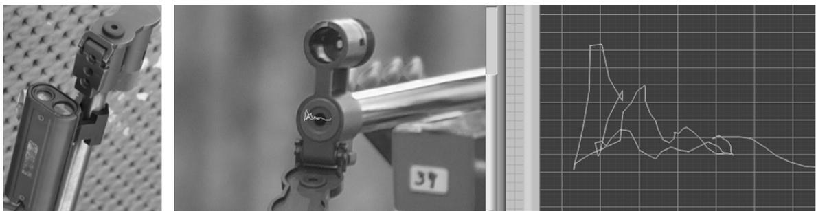
Figure 1: Left: optoelectronic feedback system Noptel. Right: video-based system. The plotted line in the diagram represents the trajectory of the muzzle obtained from the video (Baca & Kornfeind, 2006)
