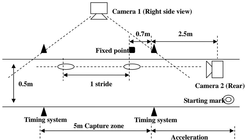
**Figure 1: Experimental set up of overground surface on field**
