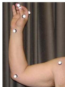
Figure 1: Reflective marker set used to track the motion of the arm and hand (posterior shoulder, lateral elbow and posterior wrist markers not shown).
