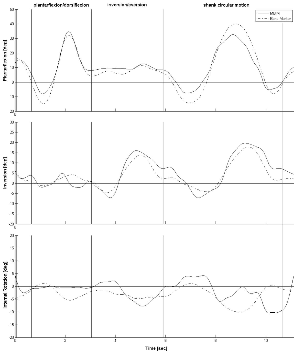
**Figure 2. Ankle joint angles of the specimen, calculated with the bone marker based motion analysis (dotted lines) and the model-based image-matching (MBIM) technique (solid lines).**
