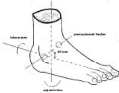
Figure 2. The position of the three axis of rotation of the ankle loading apparatus in respect of the foot and lower leg. The intersection point of the plantar-dorsal axis lies 20 mm proximal of the centrepoint between the lowest points of the medial and lateral malleoli.
