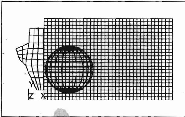
Fig. 1. The ball-foot interaction model using Eulerian and Lagrangian frames.
