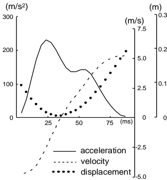
**Figure 2 - Displacement, velocity, acceleration of the ball during contact calculated from video images.**
