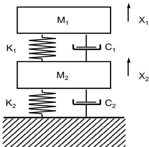
**Figure 3 - Mass-elasticity-viscosity model of**
