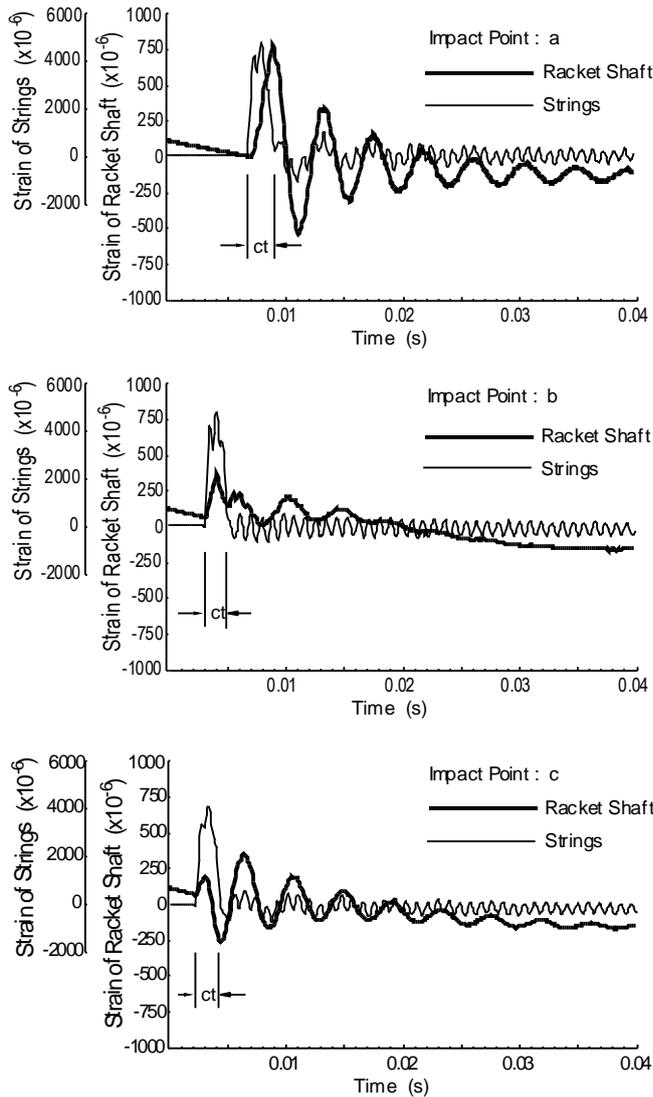
**Figure 2 – Strain of racket shaft and strings at impact point a (Top), b (Middle) and c (Bottom).**
