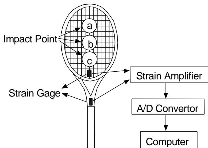
Figure 1 – Diagram of collision of rackets and balls.
