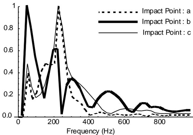
**Figure 3 – Layered frequency of racket shaft at 3 impact points.**
