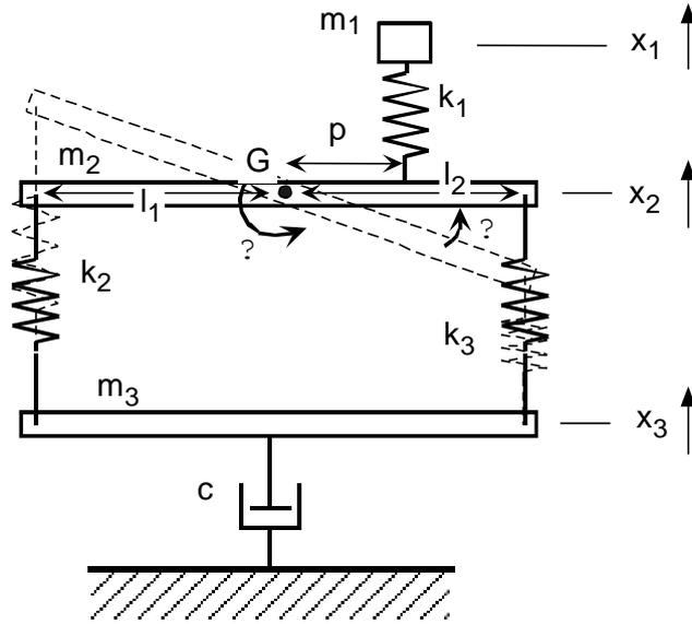
Figure 4 – Model of racket and ball.
