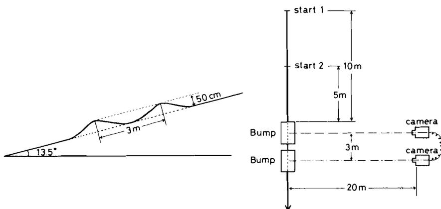
Fig. 1 Slope and bumps used for experiments 1 and 2.
