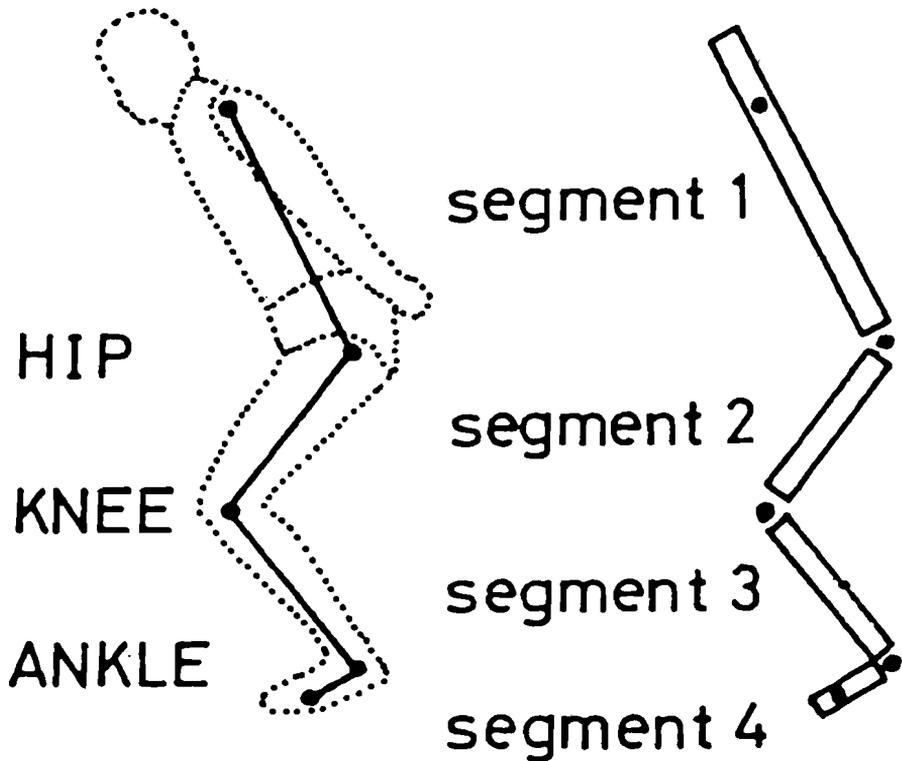
Fig. 2 Four segment link model used for mechanical analysis of experiment 2.
