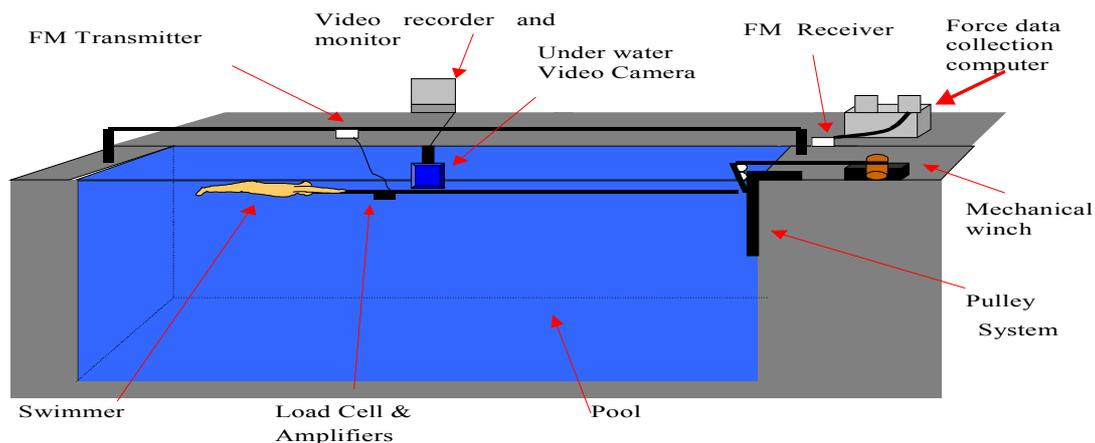
**Figure 1 - Schema of the experimental set-up for quantifying net forces.**
