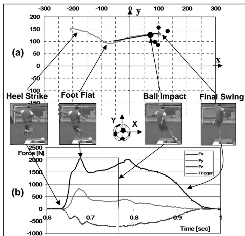
Figure 4: (a) COP trajectory for right footed player 1 HL (grey line), linear approximation of the kick phase (black line) and COP at the impact (black points: smaller point for other successful shots) referred to the force platform system. (b) Corresponding GRF plots and trigger.
