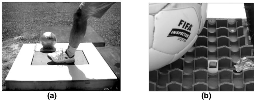
Figure 1: **(a)** Force platform embedded in the wooden runway. **(b)** Detail of the ball trigger.
