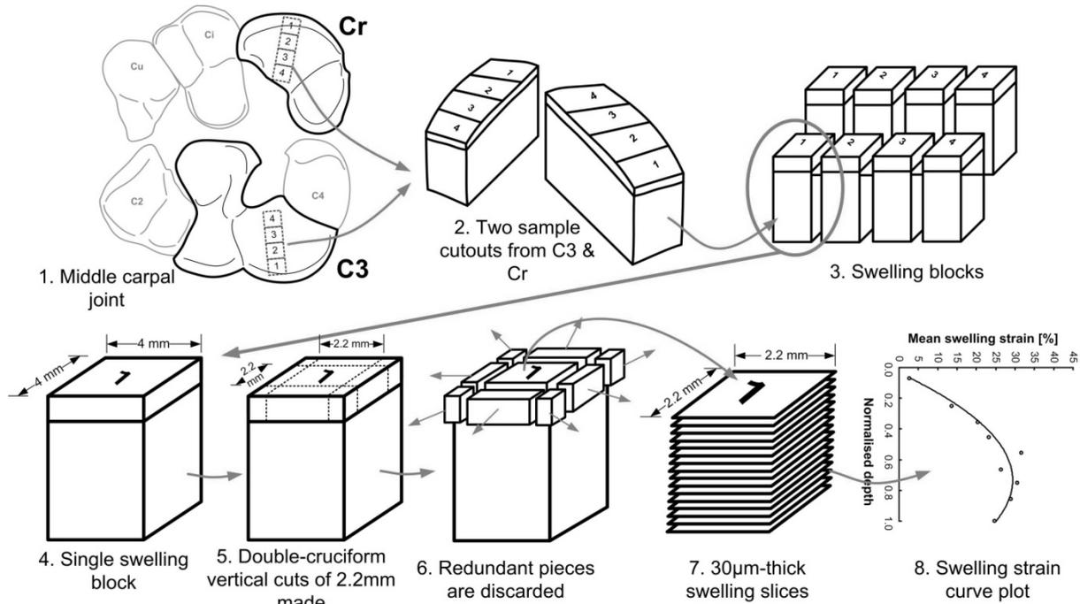
Figure 2 - Schematic showing procedure used for obtaining serial slices for the cartilage matrix free-swelling studies from the four sampling sites on the C3 and Cr surfaces.
