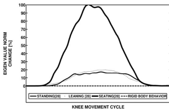
**Figure 2: Deviation from the rigid body behavior on the thigh with respect to three postures**
