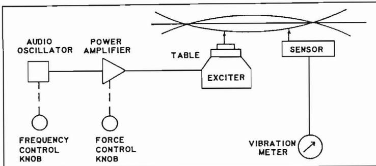
Figure 1. Vibrational measurement system.
