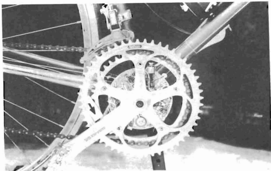
Figure 1. Instrumented crank and chain ring with one foil strain-gauge indicated by an arrow.
