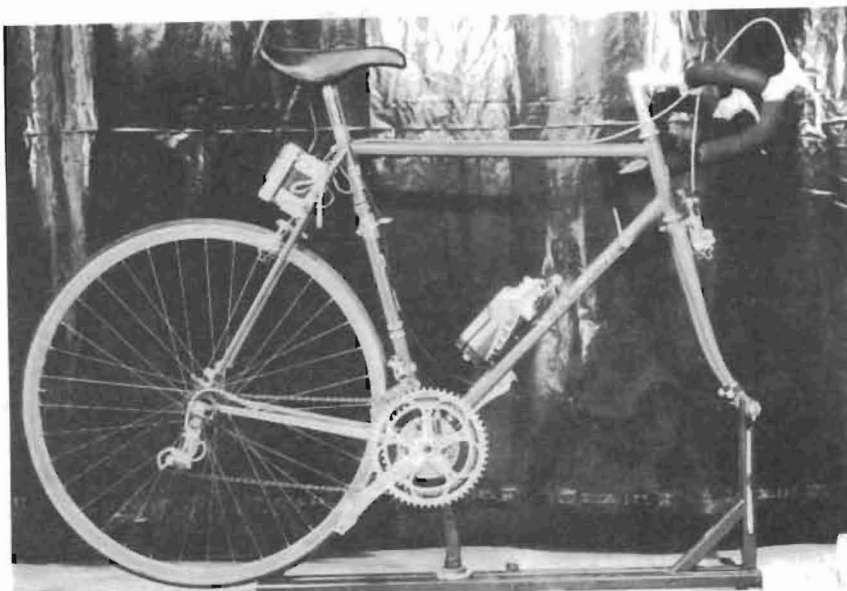
Figure 4. Frame mounted electronics housed in a standard water bottle and the FM recorder; total weight = 620 gms.
