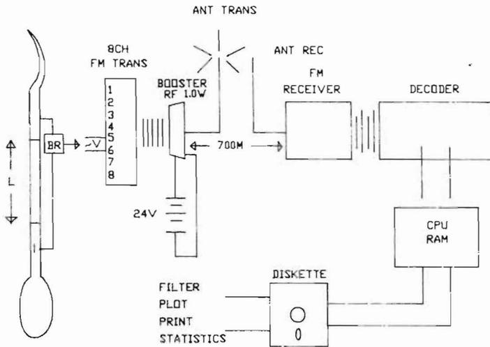
Figure 1. Stroke force measurement system schematic
