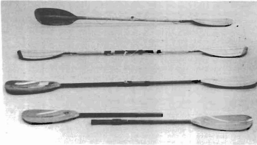
Figure 3. Instrumented kayak paddles: top - solid wood; second - wood adjustable; third and bottom - carbon fiber, adjustable, hollow core.
