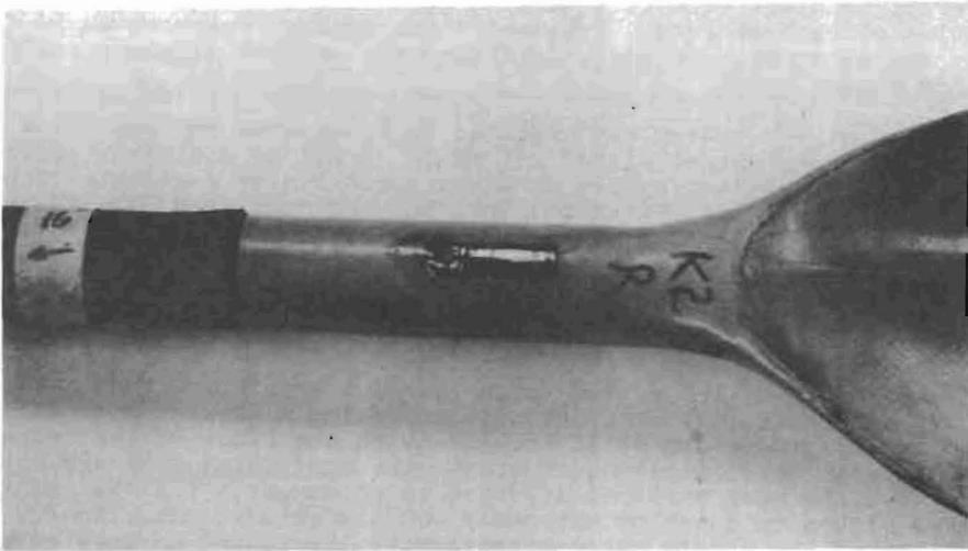
Figure 4. Strain-gauge location - kayak paddle.
