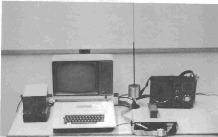
Figure 5. Signal reception, conditioning and recording instrumentation; clockwise from centre - receiving antenna, FM receiver, decoder, and microprocessor.
