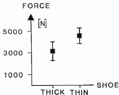
Figure 5. Comparison of impact forces with two different shoes (1 subj., 10 rep., mean, sd)
