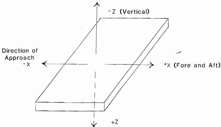
Figure 1. Force platform and identification of ground reaction forces.
