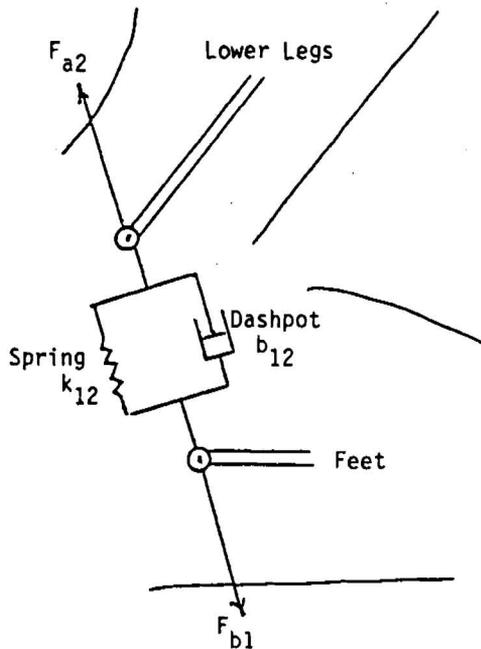
joint forces and then using them in the integration of equations 1 and 2. The method for solving these equations so that the segments remain coupled at the joints while transmitting the forces associated with the particular motion under study is outlined in the following discussion.
