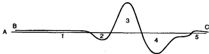
**Figure 8** Graphic portrayal of the force-deflection curves ( 1, 2, 3, 4, 5 ) for trial P6 of the Clear Backward Hip Circle to Handstand. Line "A" denotes the reference point which was the deflection of the bar when the gymnast was in the front support position. "B" denotes the top of the cast and "C" denotes the handstand position.
