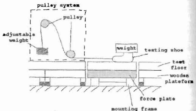
Figure 1 – mechanical slip resistance test setup
