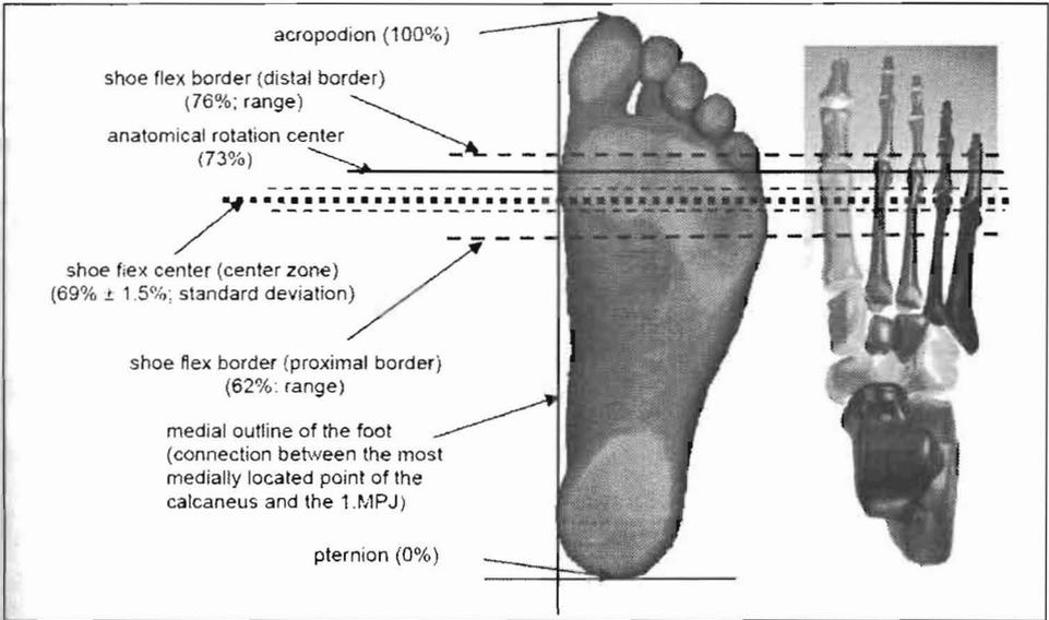
Figure 1: Construction guidelines for positioning and alignment of the transversal flex zone (not to scale).
