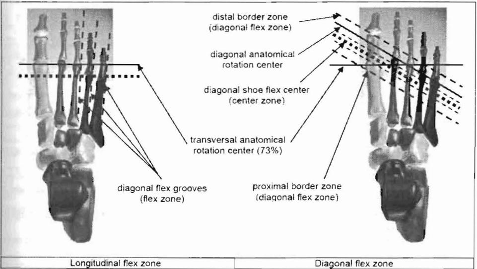
Figure 2: Construction guidelines for positioning and alignment of the longitudinal and diagonal (oblique) flex zone (not to scale).
