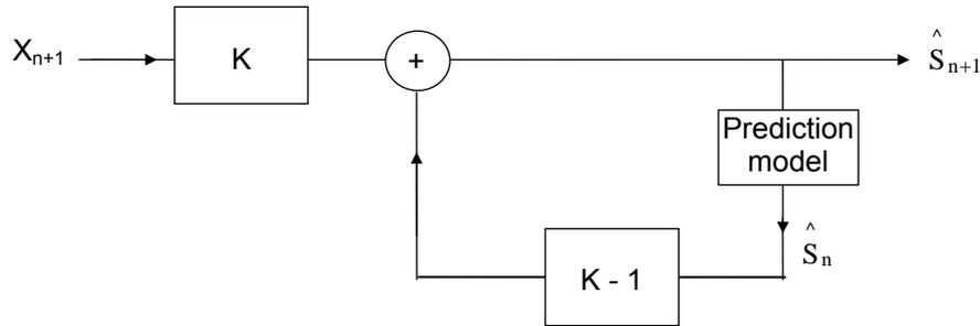
**Figure 3.** Block diagram of a simple Kalman Filter
