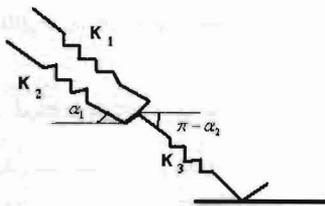
Figure 1 Leg's discrete muscle-spring Simulation.
