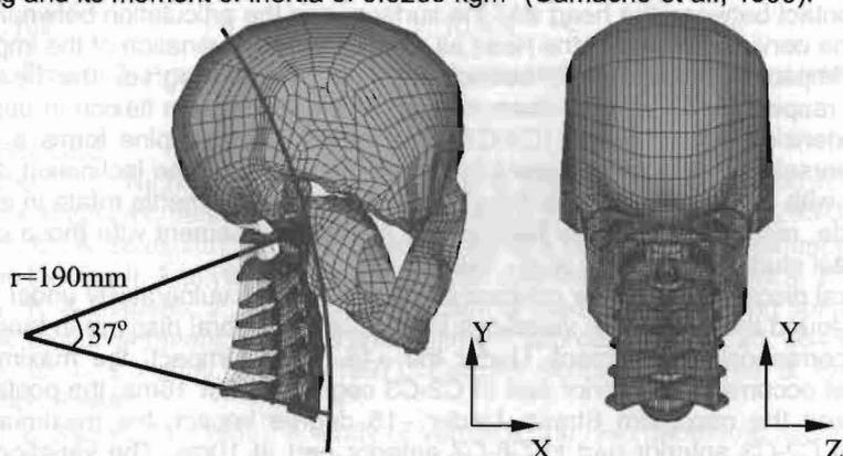
**Figure 1** Finite element mesh of the head and cervical spine model.
