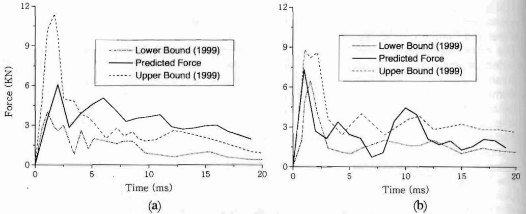
**Figure 2** Comparison of predicted resultant head impact force history against experimental data (from Camacho et al., 1999). (a) The impact orientation at  $-15$  degree (b) The impact orientation at  $+15$  degree.
