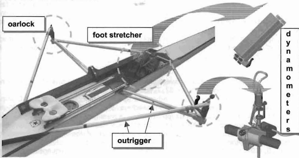
**Figure 2 Measuring the dynamics in rowing. The dynamometer for measuring reaction forces may either be attached to the foot stretcher in the boat (depicted here) or to that of the ergometer. To measure pulling forces, a pair of dynamometric oarlocks is attached to the outriggers.**
