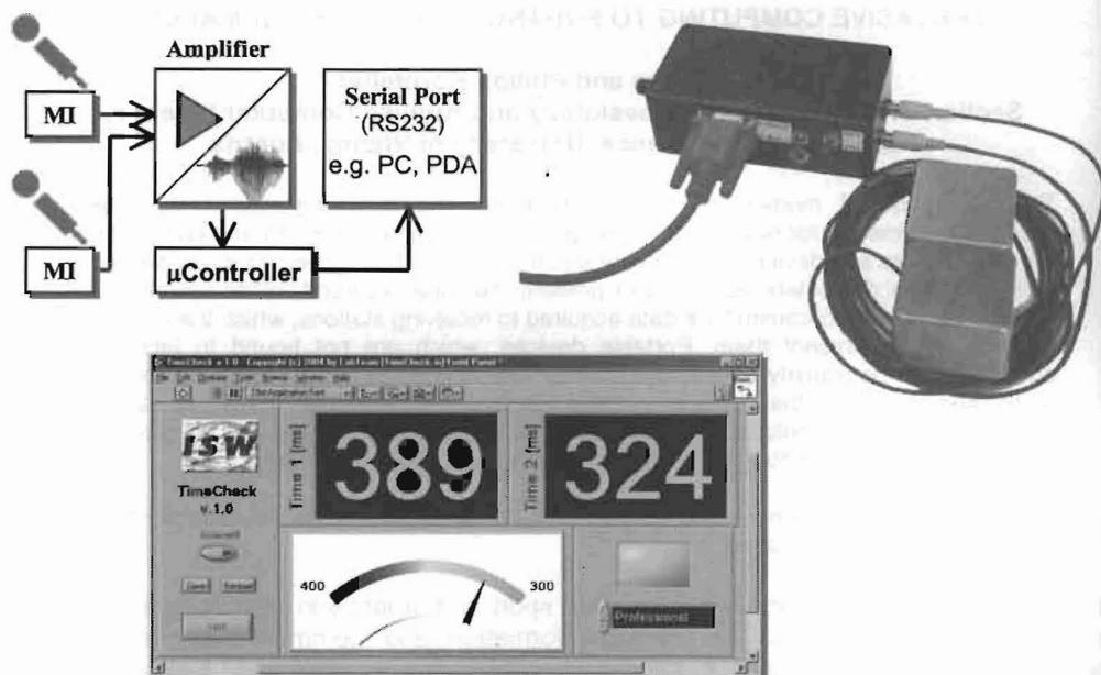
**Figure 1** Ball impact time interval detection system. Upper left: Block diagram of the measuring system. Upper right: Photo of the system. Lower: Graphical user interface (times between first and second impact as well as between second and third impact are displayed after a short table tennis serve).
