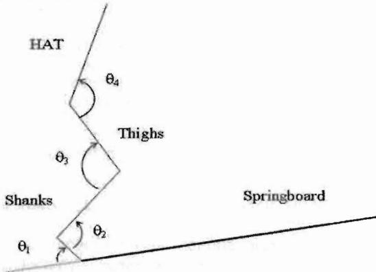
**Figure 1** Body segments and springboard are connected by frictionless revolute joints.
