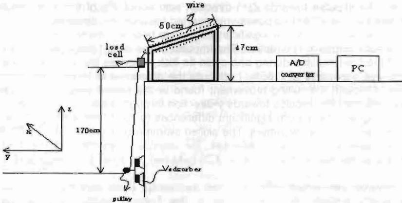
**Figure 2** The side view of the measuring system for propulsive force. The Load cell acquires data through pulley which could divert the force direction, and the data is stored to PC.
