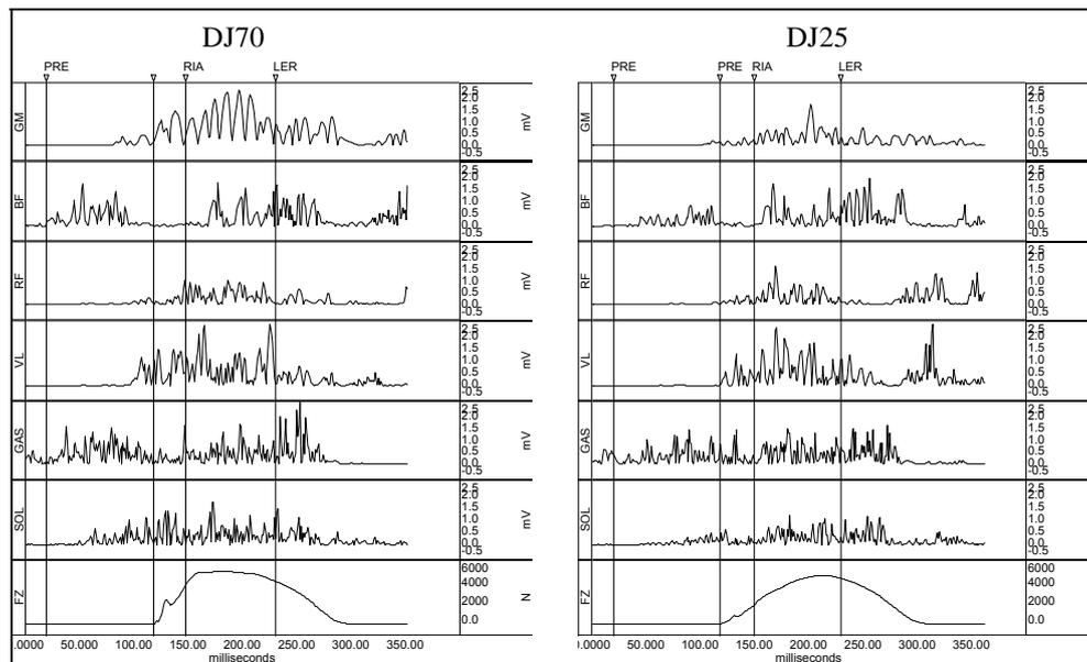
**Figure 1** - Averaged signals of force (Fz) and rectified EMG's (REMG) of gluteus maximus (GM), biceps femoris (BF), rectus femoris (RF), vastus lateralis (VL), gastrocnemius (GAS) and soleus (SOL), On the left panel DJ70 on the right pane DJ25. Note the increase of REMG on the RIA phase muscles during DJ70.
