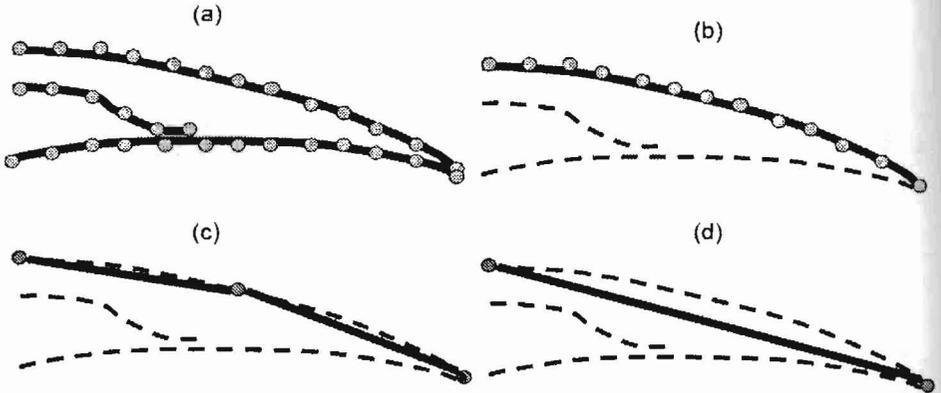
Figure 1: Models of the springboard. (a) Consist of 10cm length rigid segments. (b) Twelve segment model consist of upper board only (c) Two segment model consist of upper board only (d) One segment model consist of upper board only.
