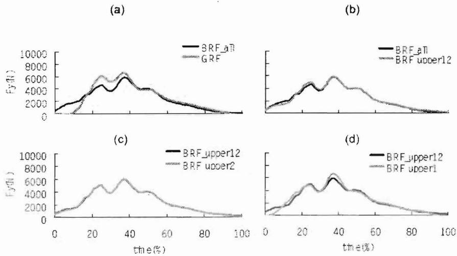
Figure 2: Reaction force. (a) The board reaction force calculated from 29 segment model (BRF\_all) and the ground reaction force (BRF). (b) BRF\_all and the board reaction force calculated from 12 segment model consist of upper board only (BRF\_upper12). (c) BRF\_upper12 and the board reaction force calculated from 2 segment model consist of upper board only (BRF\_upper2). (d) BRF\_upper12 and the board reaction force calculated from 1 segment model consist of upper board only (BRF\_upper1).
