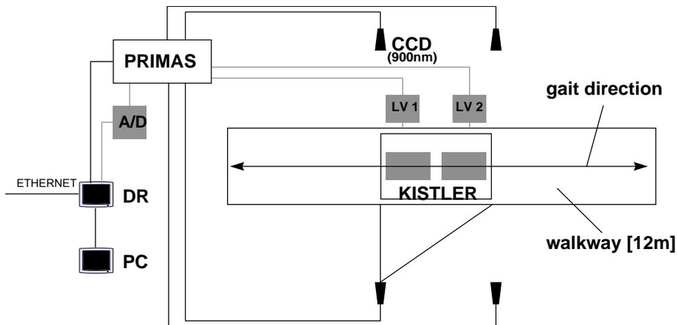
**Fig. 1:** Principle of the used gait lab (LV1,2: Force plate amplifiers; A/D: Analog-Digital-Converter; DR: Measuring computer; PC: Computer for data processing)
